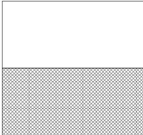
Figure 18. Schematic diagram of the mixed phase initialization (MPI). The (complete) ordered initial state in the upper side and a random initial state in the lower side are merged.
